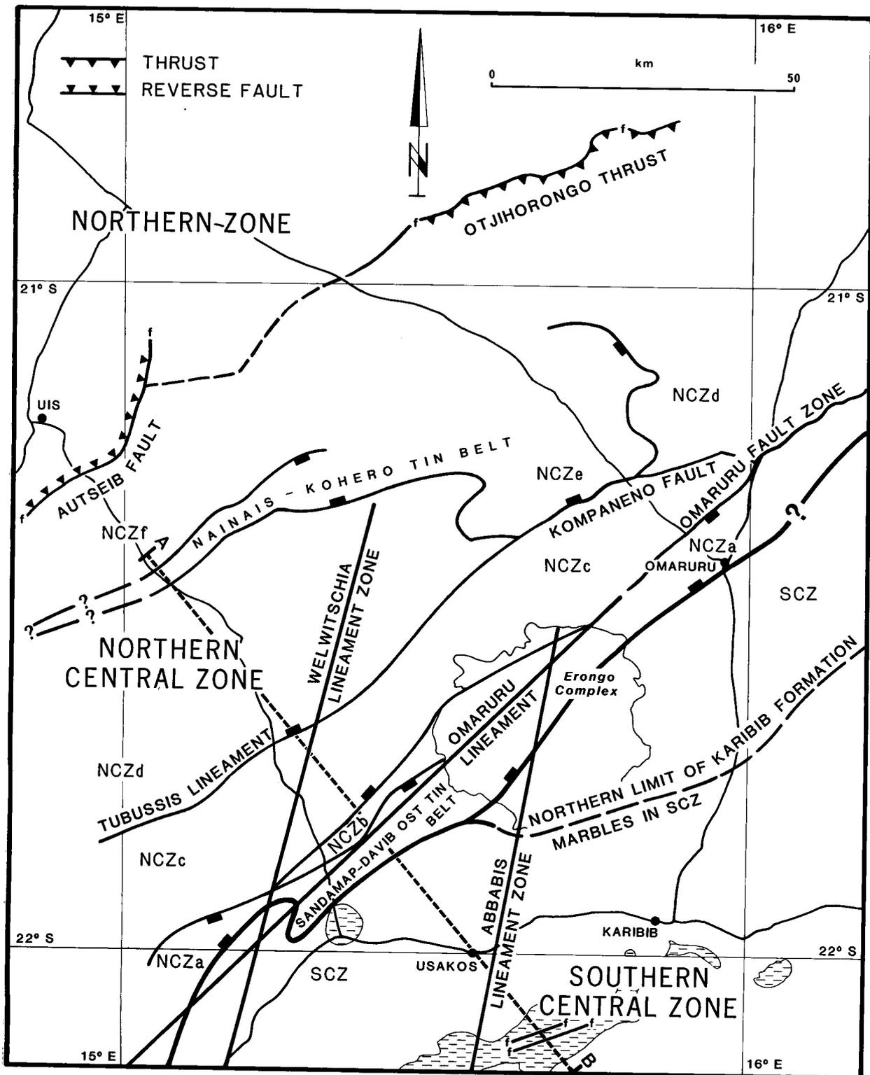
**Figure 2.4:** Tectonostratigraphic zones of the Usakos—Karibib—Omaruru area (modified after Badenhorst, 1987). Block on side of fault/lineament that on aggregate was downthrown during Damaran sedimentation. A-B marks section line shown in Figure 2.5
