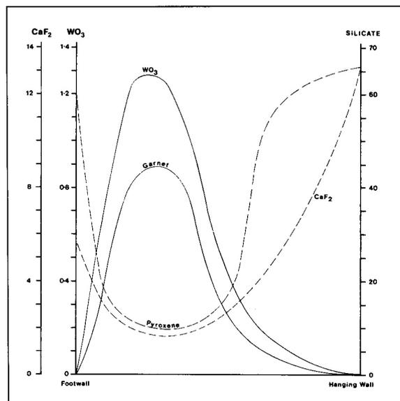
**Figure 7/3.3:** Schematic diagram showing mineralogical zonation and variations in wt%  $\text{CaF}_2$  and wt%  $\text{WO}_3$  contents across garnet-facies skarn (after Steven, 1987)
