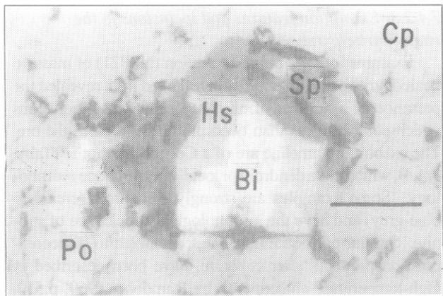
Plate 7/4.3: Bismuth (Bi), hessite (Hs), sphalerite (Sp) and pyrrhotite (Po) aggregates in massive chalcopyrite (Cp) ore from Onguati Copper Mine (NSP21; RL); scale bar = 50 µm
