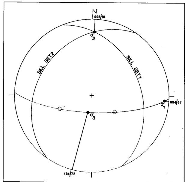
**Figure 4.2:** Conjugate pegmatite sills in the Abbabis Inlier and the theoretical stress field under which similarly oriented fractures would develop
