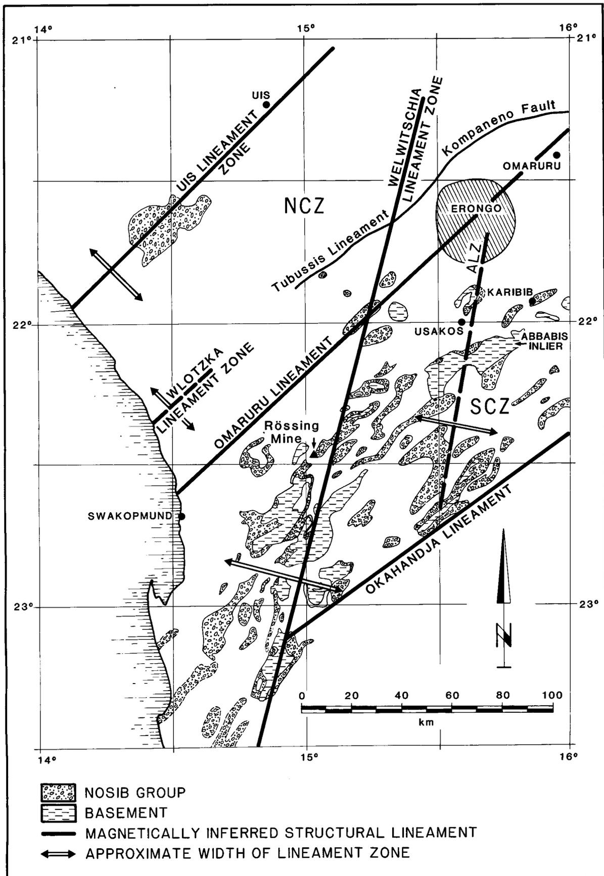
Figure 2.3: Structural lineaments and exposures of basement inliers and Nosib Group metasediments in central Namibia (modified after Corner, 1983)
