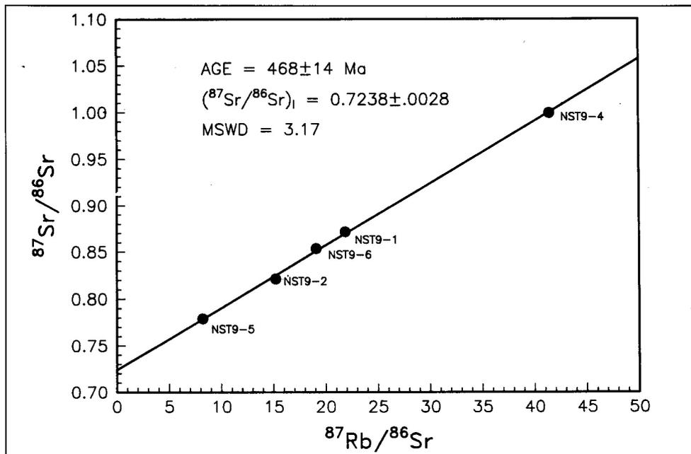
Figure 6.7: Rb-Sr whole-rock isochron for stanniferous pegmatite from Sandamap Tin Mine
