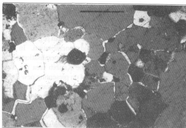
**Plate 7/4.1:** Granoblastic quartz in chalcopyrite-pyrrhotite (opaque phases) skarn from Onguati Copper Mine (NSP18; XL); scale bar = 0.5 mm
