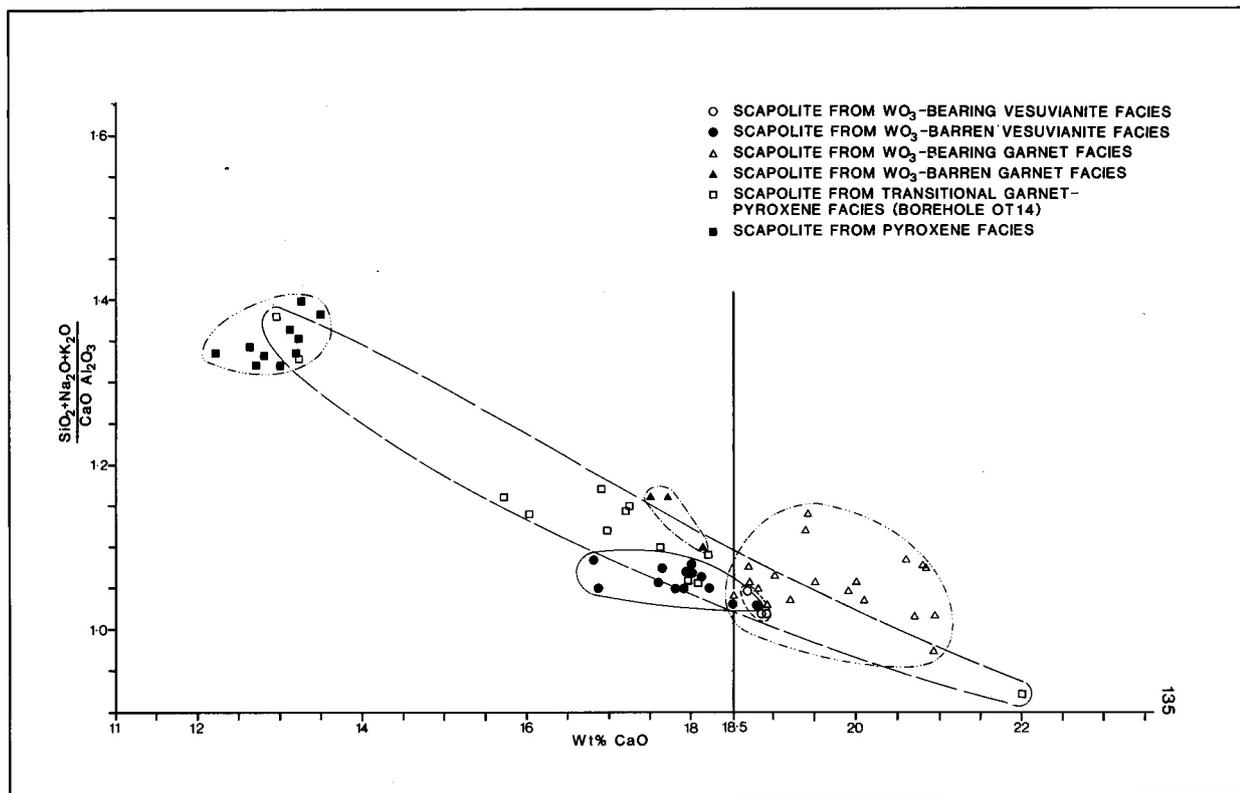
Figure 7/3.4:  $(\text{SiO}_2+\text{Na}_2\text{O}+\text{K}_2\text{O})/(\text{CaO}+\text{Al}_2\text{O}_3)$  versus wt% CaO for skarn scapolite analyses (after Steven, 1987)
