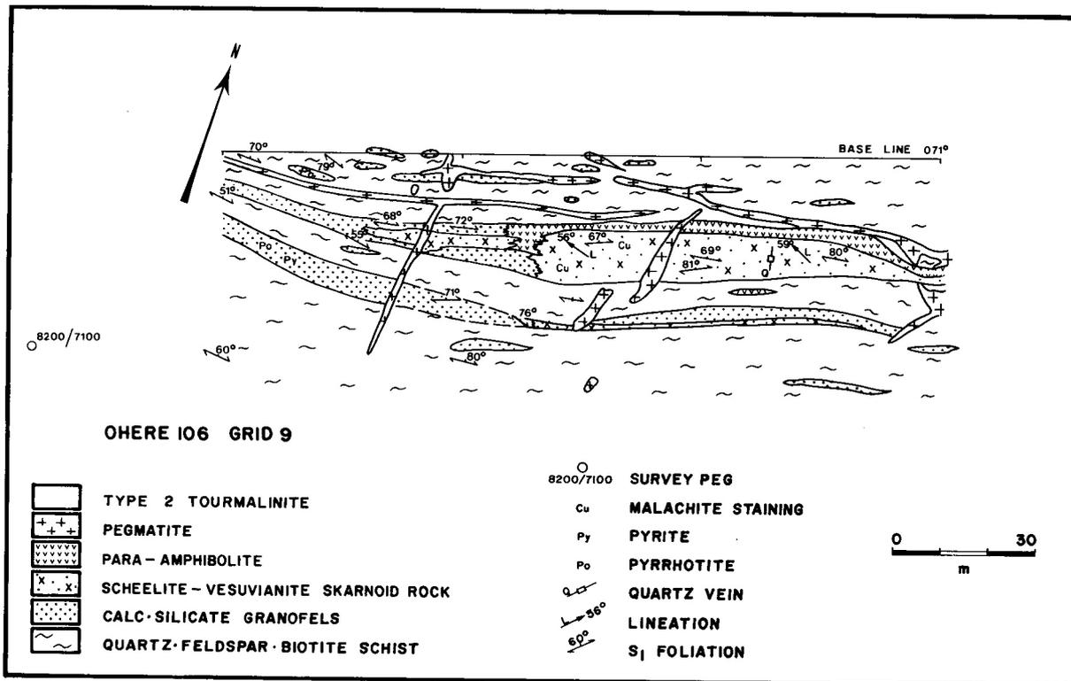
Figure 7/7.1: Geological map of scheelite-vesuvianite skarnoid rocks on Ohere 106 (grid 9)
