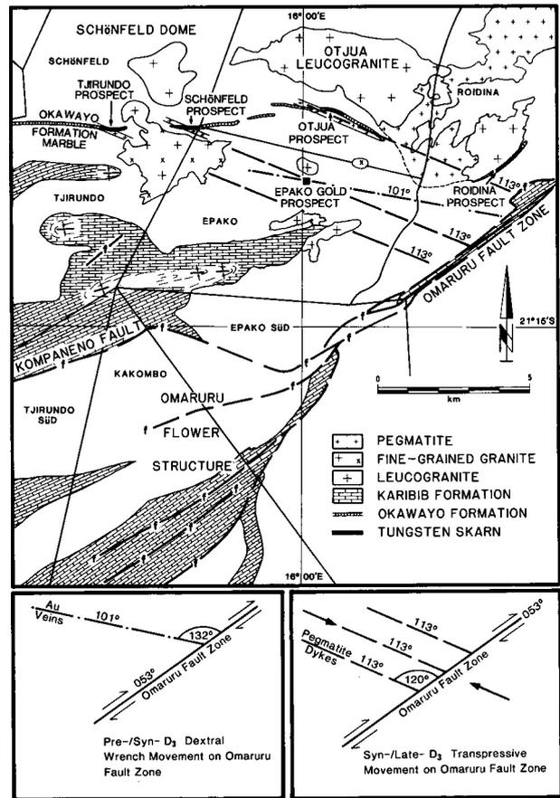
Figure 4.4: The relationship between dextral movement on the Omaruru fault zone, granitic intrusion and mineralisation in the Schönfeld Dome
