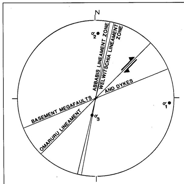
**Figure 8.2:** Principal stress axes during D<sub>4</sub> deformation in the SCZ. Note dextral motion on Omaruru Lineament
