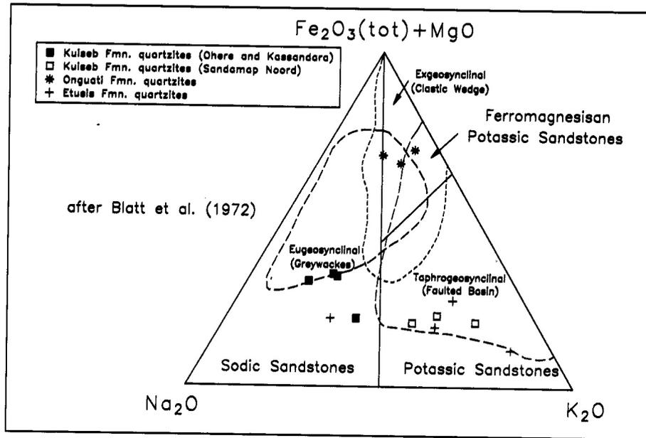
Figure 2.9: Chemical composition of CZ quartzites in relation to tectonic setting
