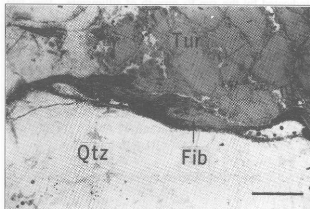
**Plate 5.4:** Fibrolite (Fib) segregation rimming zoned tourmaline (Tur) in sheared pegmatite, immediate vicinity of gold mineralisation, Sandamap Noord Gold Prospect, trench 22 (SN302; PPL); scale bar = 1 mm
