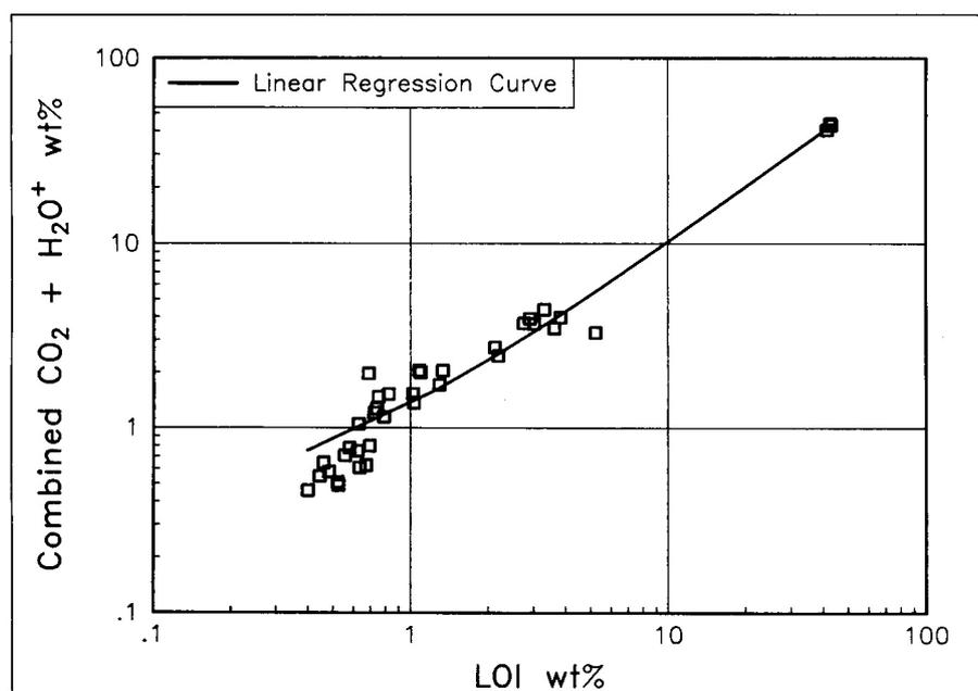
Appendix Figure 1: Combined CO<sub>2</sub> + H<sub>2</sub>O<sup>+</sup> (GS) vs LOI (UCT)
