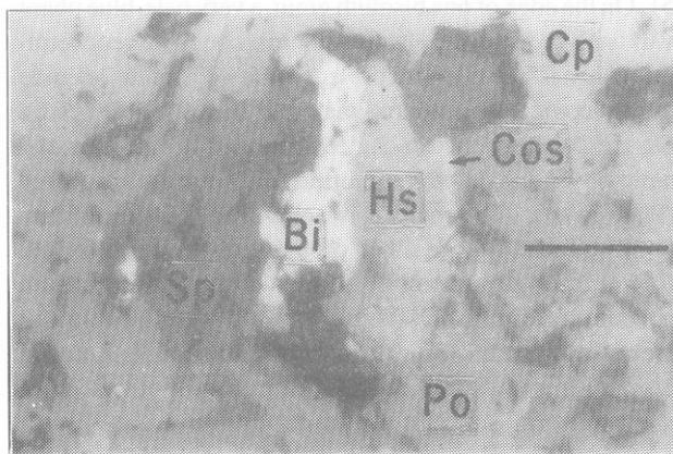
Plate 7/4.4: Bismuth (Bi), hessite (Hs), sphalerite (Sp), costibite (Cos) and pyrrhotite (Po) aggregates in massive chalcopyrite (Cp) ore from Onguati Copper Mine (NSP21; RL); scale bar = 50 µm
