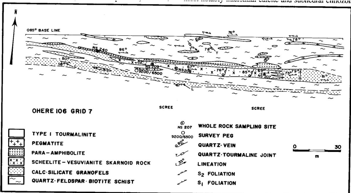
Figure 7/7.2: Geological map of scheelite-vesuvianite skarnoid rocks on Ohere 106 (grid 7)
