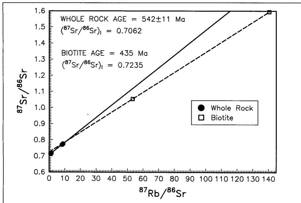
Figure 6.8: Rb-Sr isochrons (WR and minerals) for the Ohere Oos Salem granite
