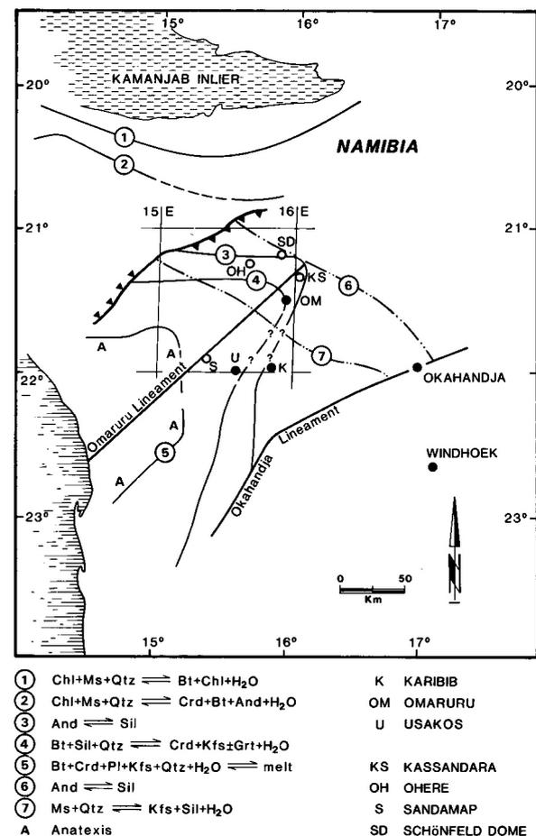
**Figure 5.1:** Isoreactiongrads in pelitic rocks in the Damaran Orogen (after Hoffer, 1977). Lower and upper sillimanite zones after Miller (1983a)
