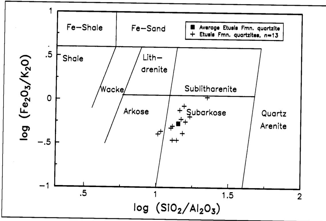
Figure 2.7: Geochemical classification of Etuis Formation quartzites at Navachab
