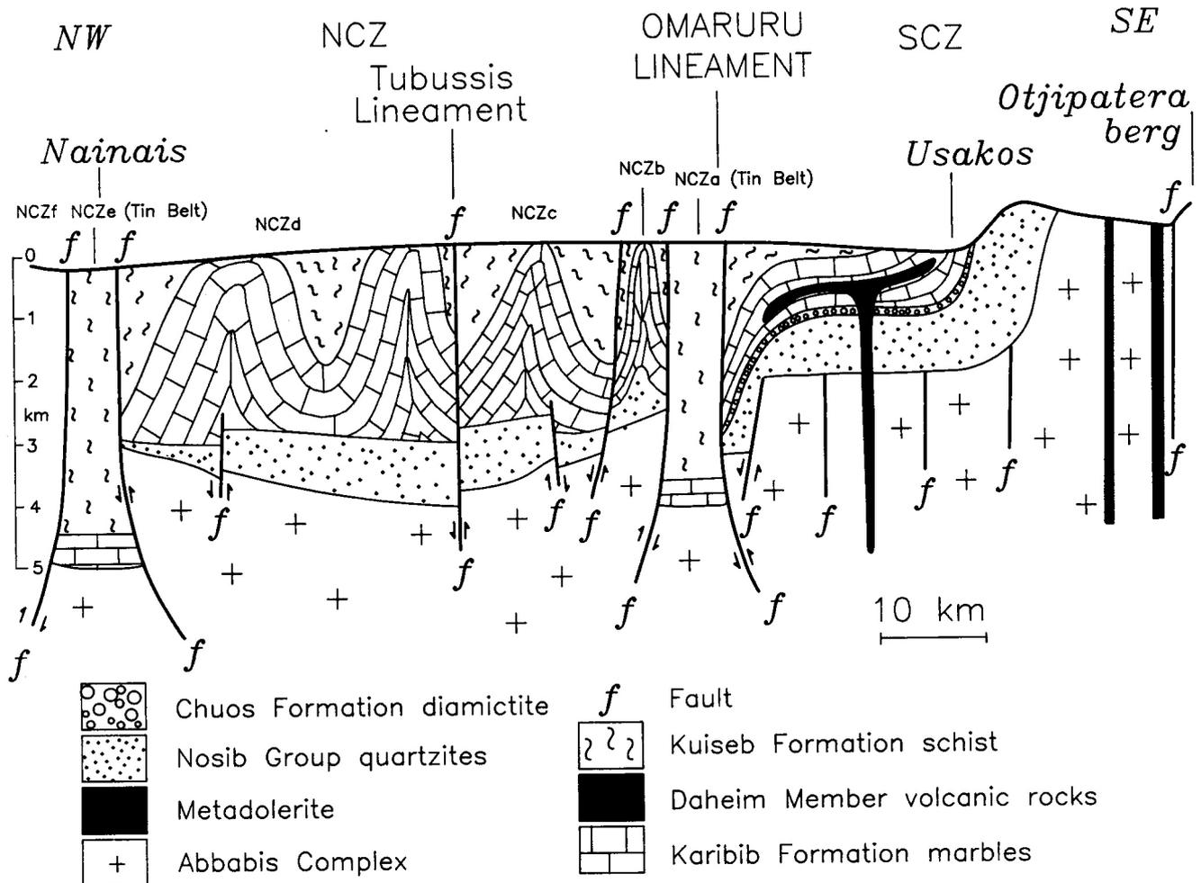
**Figure 2.5:** Schematic cross-section through the CZ showing monoclinial downfold across Omaruru Lineament. Basement profile and thickness of Nosib Group in NCZ taken from Corner's (1983) computer-model section. Granitoids have been omitted
