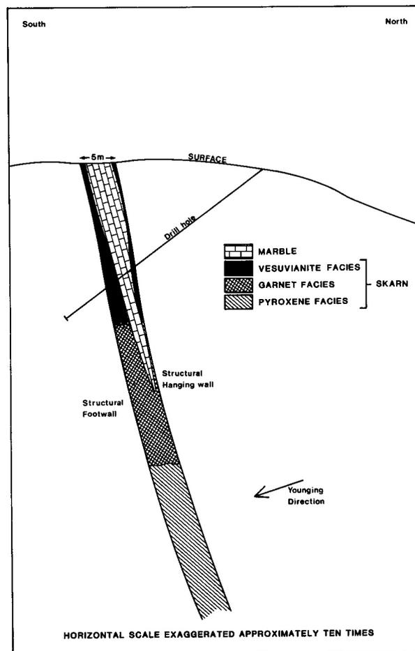
**Figure 7/3.2:** Schematic cross section through the Otjua Prospect showing direction of drillholes, overturning of sequence and varying degree of replacement of Okawayo Formation marble by skarn (after Steven, 1987)
